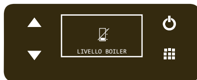
BOILER FILL TIME-OUT ALARM
