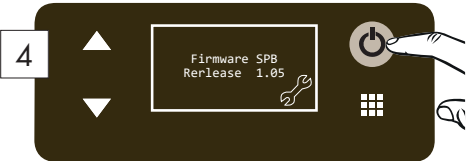
While holding the button from step 2, power on the product by setting the switch to position 1. Check that the following sequence appears:
